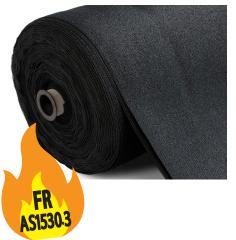
**ALLPRO**<sup>™</sup> Plus 95 FR is a superior quality 95% commercial grade shadecloth, suitable for architectural use. It is lightweight (235gsm) to allow easy tensioning, and has been heat set to prevent curling and enable easy fabrication. This also creates a superior looking end product that should not stretch or sag. Plus 95 FR has the added feature of being fire retardant for enhanced safety.
