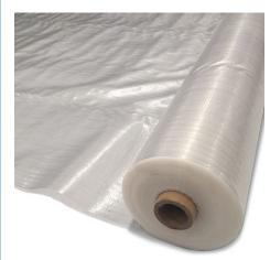
**Abshade**<sup>™</sup> Solarshield Hortcover is a reinforced greenhouse film. The reinforced cover consists of thin strips of clear plastic, woven together to make a sheet, similar to a woven weed matting (but clear). This resultant sheet is then laminated with a thin layer of plastic on each side.
